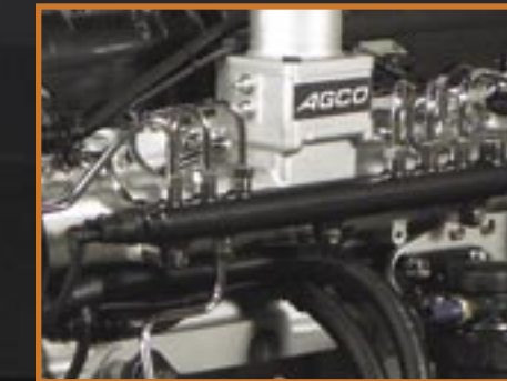
EEM3 also controls the fuel lubricated 3-cylinder radial plunger pump, and features a 20,000 psi high-pressure, common rail injection system.
