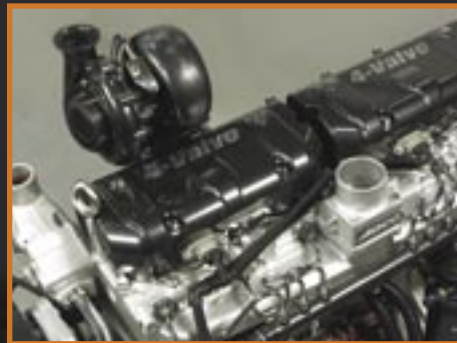
24-valve head design for improved air-to-fuel mix, reducing emissions and improving fuel consumption.
